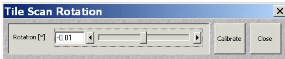
**Calibrate** - Automatically finds the rotation angle between the scanners and the stage axis.
