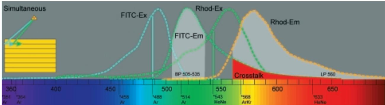
Classical simultaneous excitation and detection of fluorescence FITC/Rhodamine
