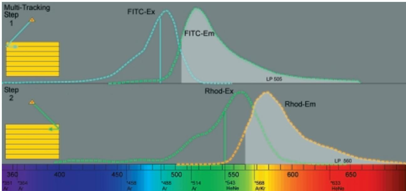
*Multi-Tracking: Separate excitations – separate detection
